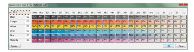
Initially it is required to read the fabric color. Afterwards it is necessary to read the stripes of colors (in everything 24 color chips). The procedure is performed pressing the key of reading of the spectrophotometer after having positioned it on the color chip. If a wrong color was read, it is possible to select it with thw mouse and read it one more time.
