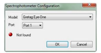
To configure the spectrophotometer it is necessary to connect the tool: the type of connection of the computer depends on the model (usually USB or serial). Subsequently choose the name corresponding to the model in the available list. If the operation is correct the LED in the window will appear of green color. Otherwise it is possible to try to change the number of connection port.
